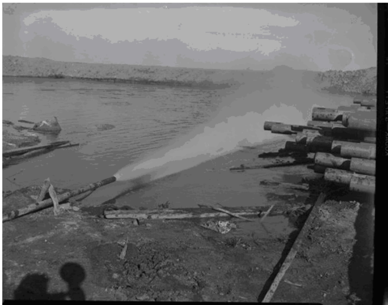
A natural gas well being 'blown down' into a pit - note the fluids, sand, water, and wastes fall into the pit - and the methane escapes to the atmosphere. What are the environmental or safety issues an operator should be concerned with?
