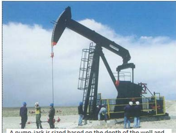
A pump-jack is sized based on the depth of the well and the expected fluid volumes. Many wells produce both crude oil and produced water, with the water making up the majoring of the fluid stream. Some can get quite large - and will interfere with irrigation equipment
